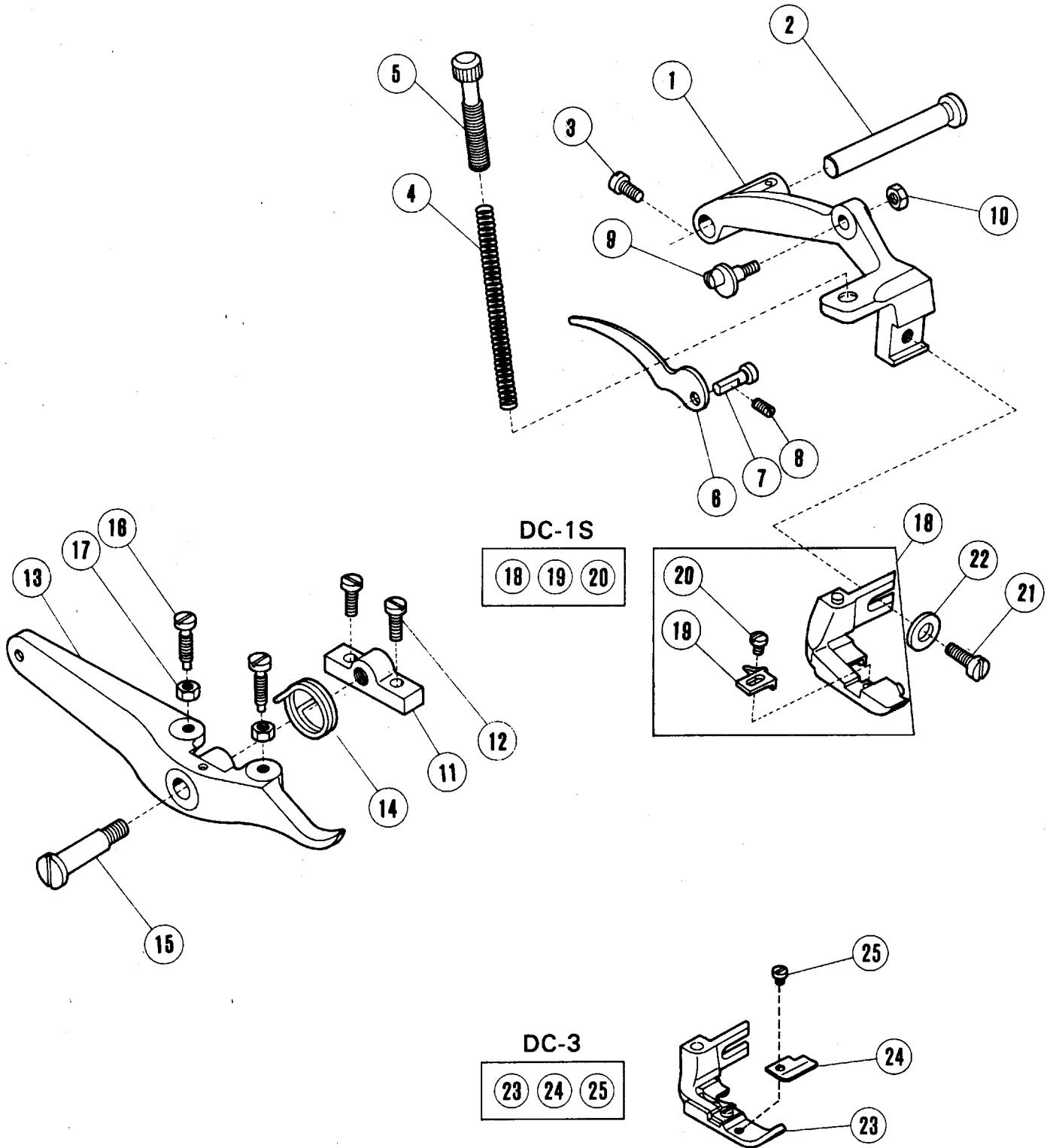
**PRESSER FOOT & LIFTING MECHANISM**
